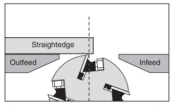
**Figure 9.** Using a straightedge to align outfeed table height with knife at TDC.
